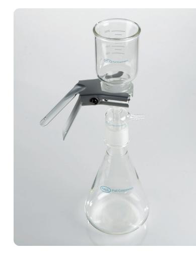
Figure 2: Glass mobile phase filtration apparatus
