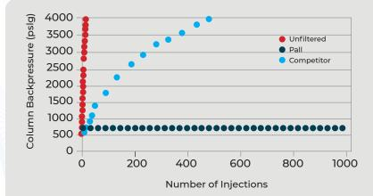
Effects of filters on HPLC column life following injections of unfiltered and filtered 0.05% latex sphere suspensions(1). With unfiltered samples, the column failed due to plugging after 19 injections. Samples passed through Competitor filters plugged the columns after 500 injections. No increase in backpressure was observed after 1000 injections of samples filtered with Pall Acrodisc® One syringe filters.
