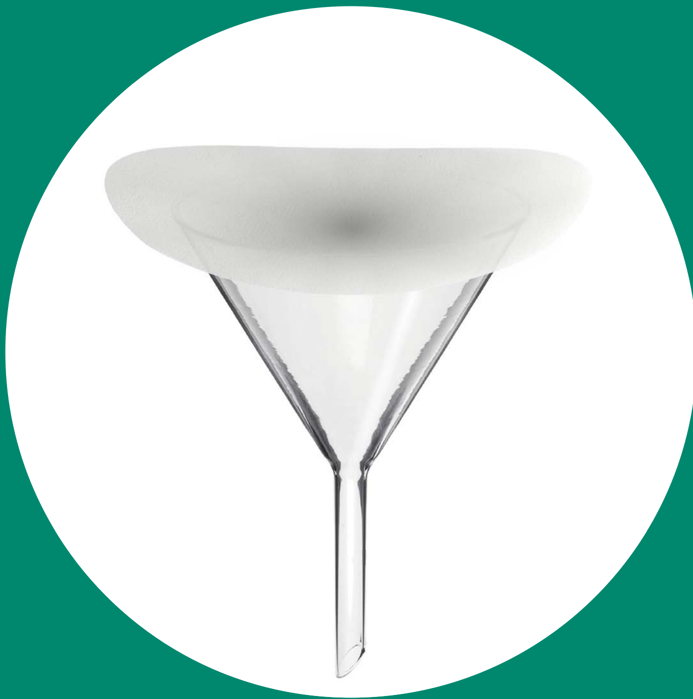
Fig 2. Glass fiber filter paper resting on top of filter funnel as specified in ASBC method Wort-9.
